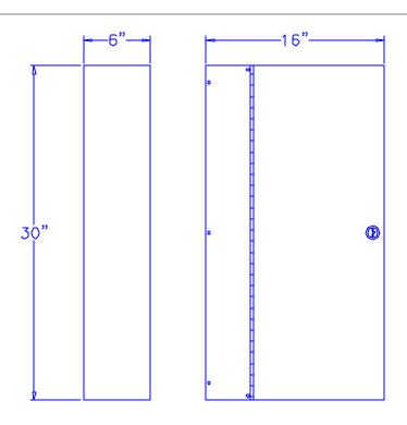
TYPICAL CABINET PAINTED, COLD ROLLED STEEL WITH HINGED, LOCKABLE DOOR
